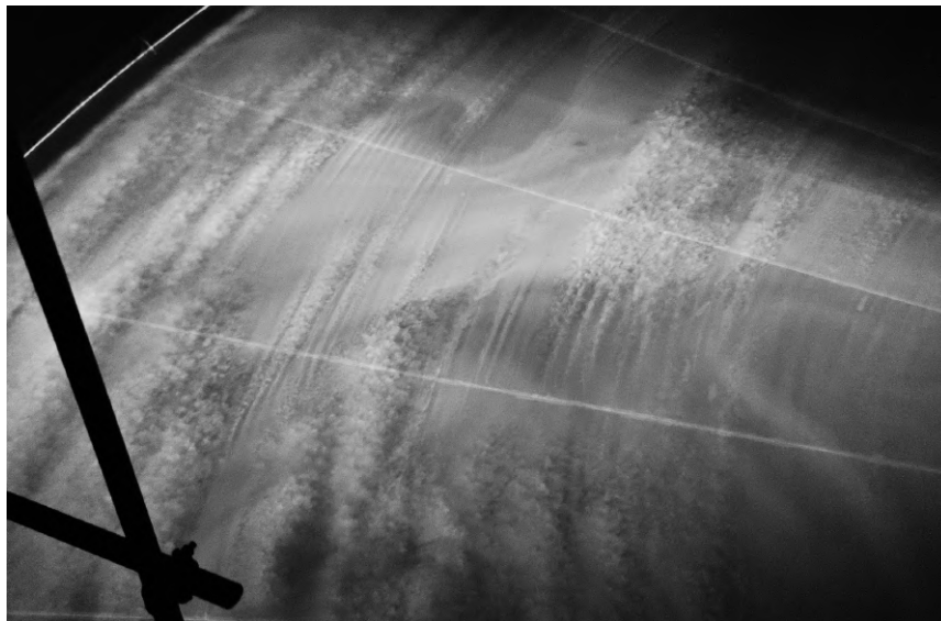
Figure VI.1: Picture of Ekman instability highlighted by dye during spin up experiment.
