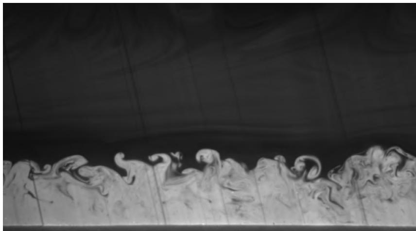
Figure II.8: Picture of a coloured layer with dye. The experiment is a spin-up in a rotating frame. The bottom is the Coriolis floor. The observed field is 35 cm in the x-axis and 26cm in the y-axis
